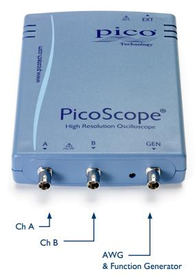
The front panel of the PicoScope 4262 has two BNC input channels and a BNC output for the function generator and AWG.
