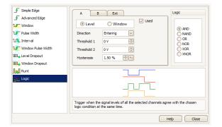
As well as the standard range of triggers found on all oscilloscopes, the PicoScope 4262 offers a comprehensive set of advanced digital triggers including pulse width, windowed and dropout triggers to help you capture the data you need.
