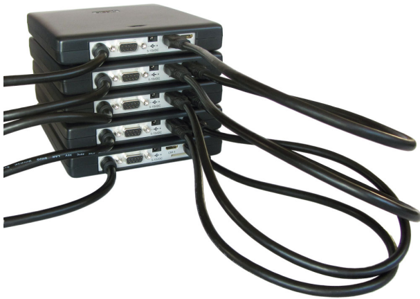
Figure 6.3: Multiple Handyscope HS6 DIFFs combined
