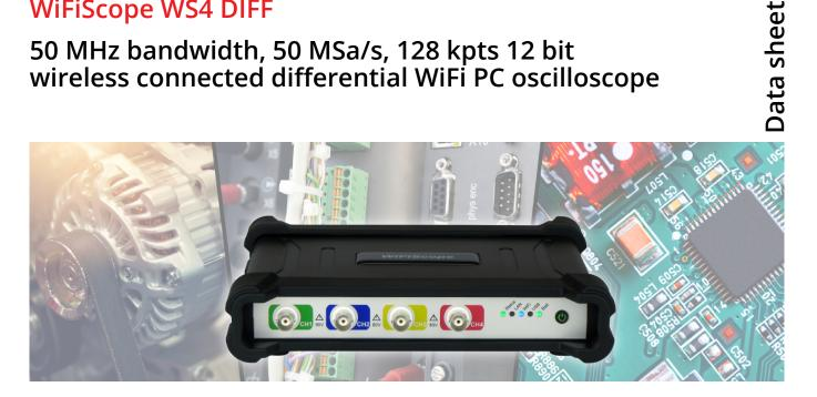
The high resolution WiFi oscilloscope with the lowest noise and high sensitivity with 4 differential input channels and 128 thousand point record length that can be filled with a sample rate of 50 MSa/s. This is the a powerful, portable, battery powered and versatile WiFi PC oscilloscope, high resolution multimeter and more..., with a universal connection through WiFi, wired LAN and SuperSpeed USB 3.0.
